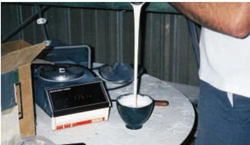
Each formula the binder and refractory manufacturing company mixes has to be tested for pour time, set time, and slump before being approved for packaging.
