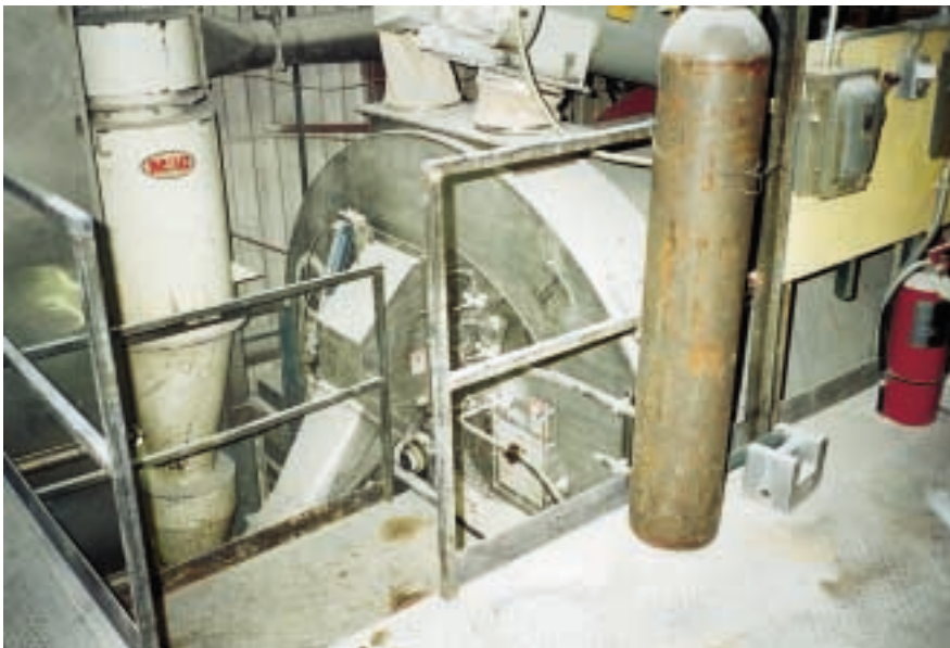
The inlet chute is at the top center of the mixer's front hood assembly and the discharge chute is on the front hood assembly's face just beneath the inlet chute.
